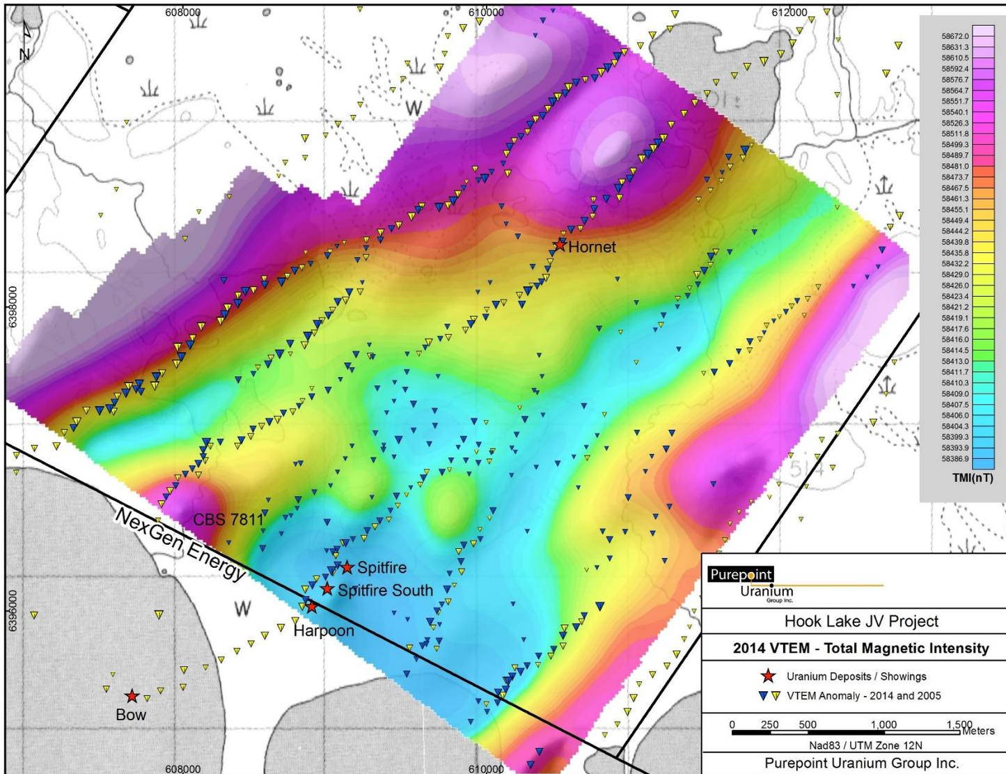
Figure 16: Total Magnetic Intensity – 2014 VTEM Survey
