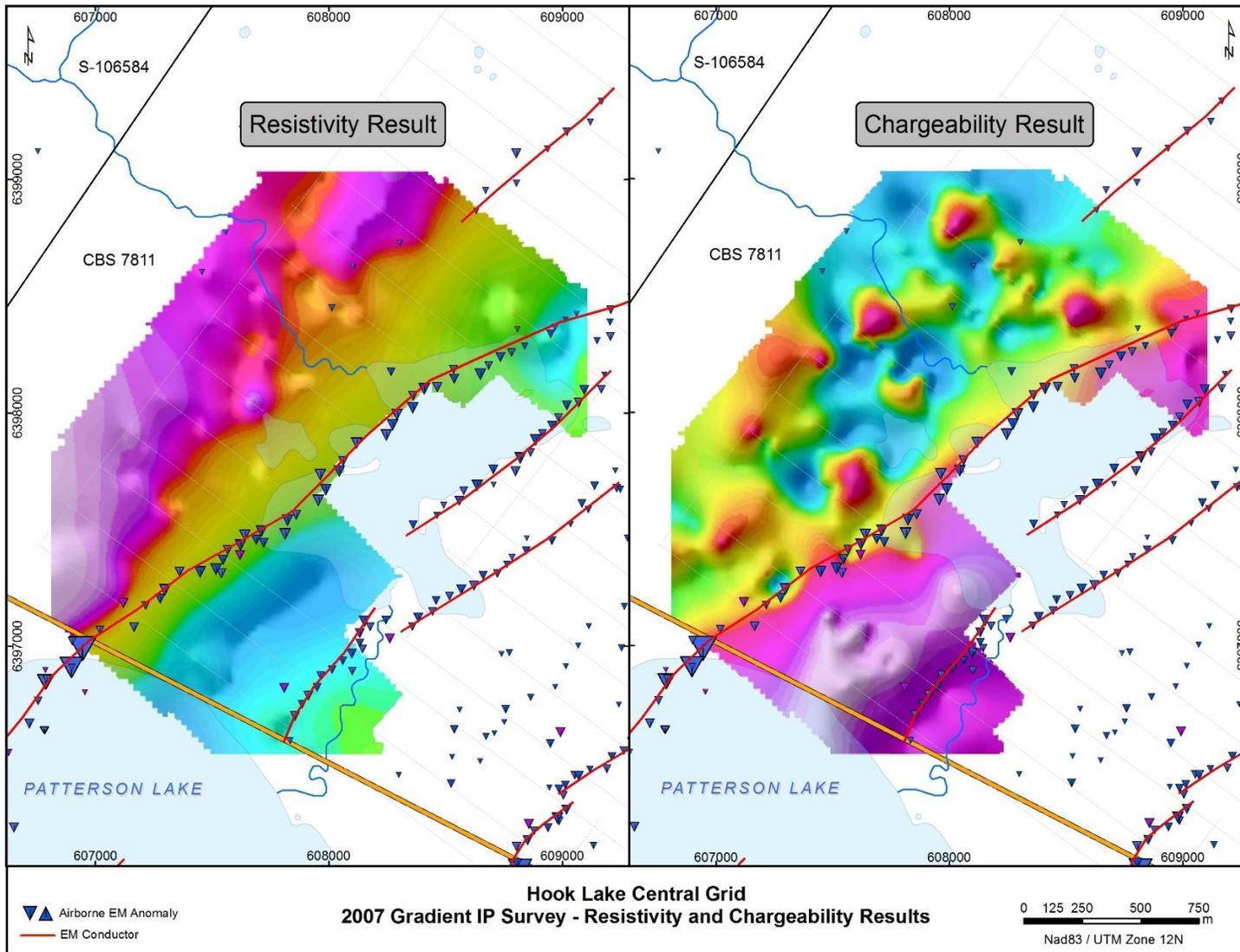
**Figure 22: Gradient Induced Polarization Results - Central Grid**
