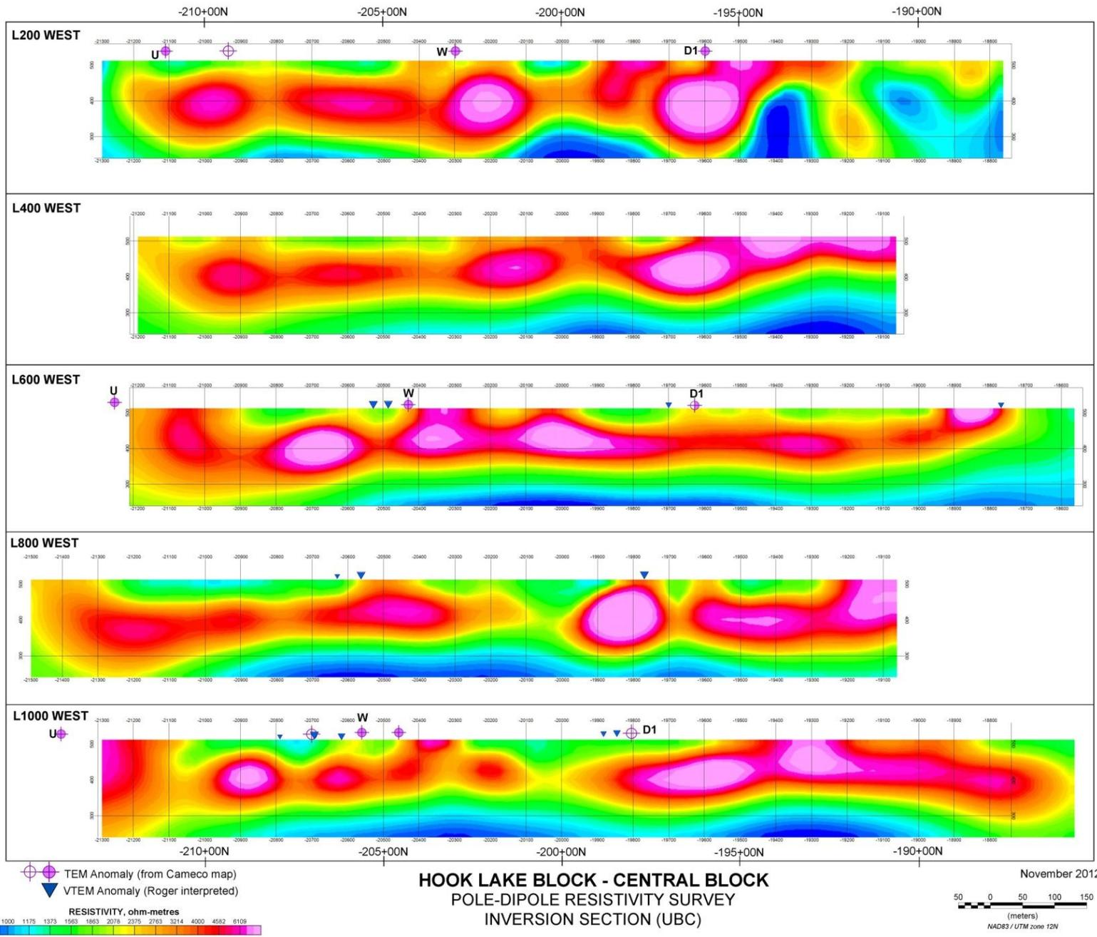
Figure 23: Stacked Pole-dipole Induced Polarization Sections - Central Grid
