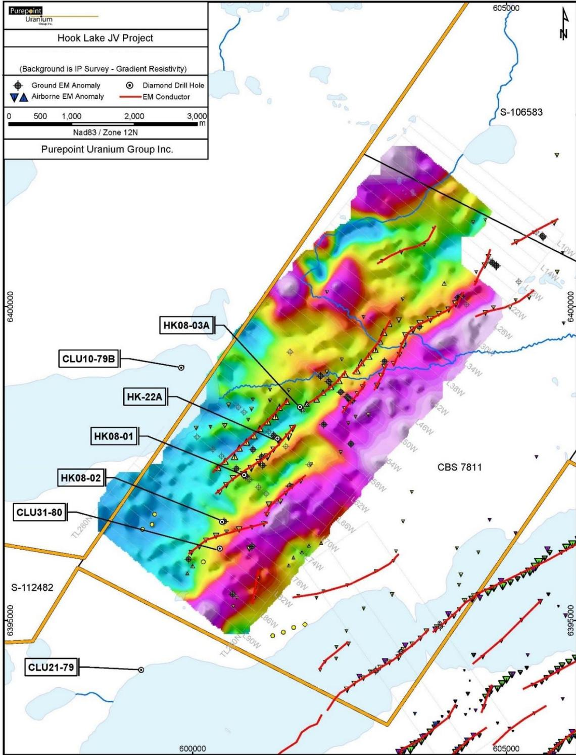
Figure 20: Gradient Resistivity Results – Carter Corridor
