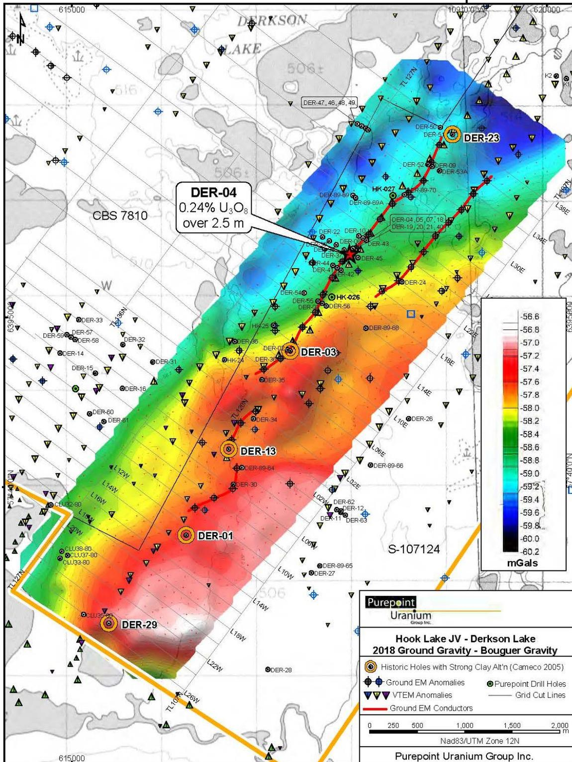
Figure 25: Bouguer Gravity Results – Derkson Area
