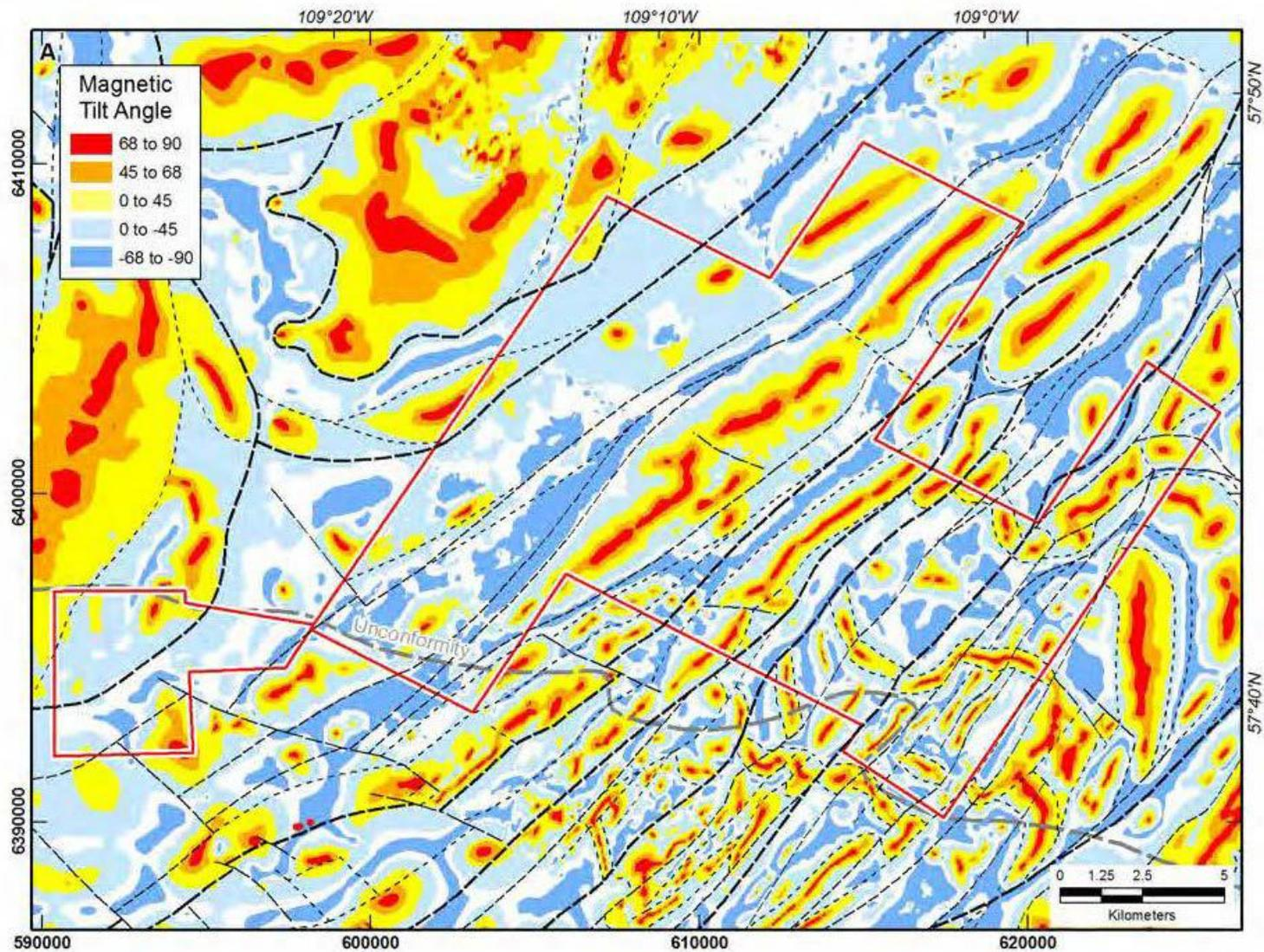
Figure 14: Magnetic Tilt with Structural Interpretation (Condor, 2013)
