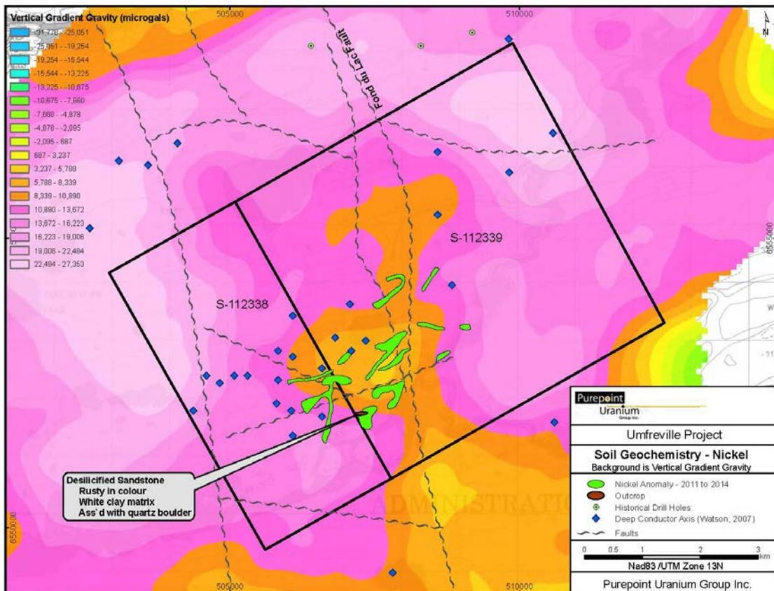
Figure 17: Nickel Soil Anomalies with Gravity Background
