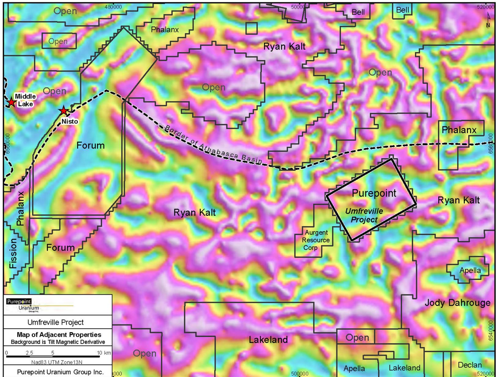
Figure 22: Adjacent Properties with Airborne Magnetics – Tilt Derivative
