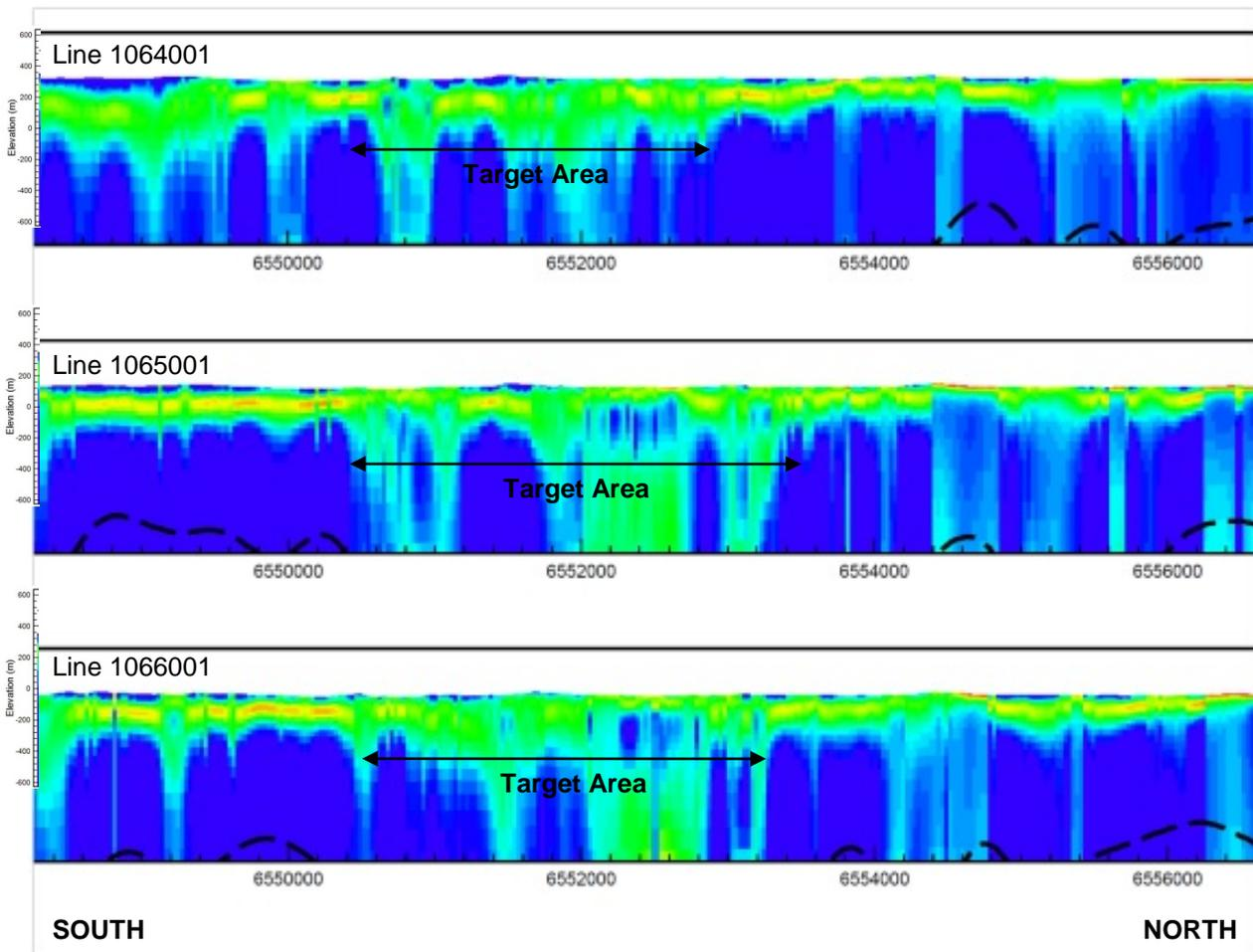
Figure 10: Example of REI Resistivity Section showing Umfreville Target Area
