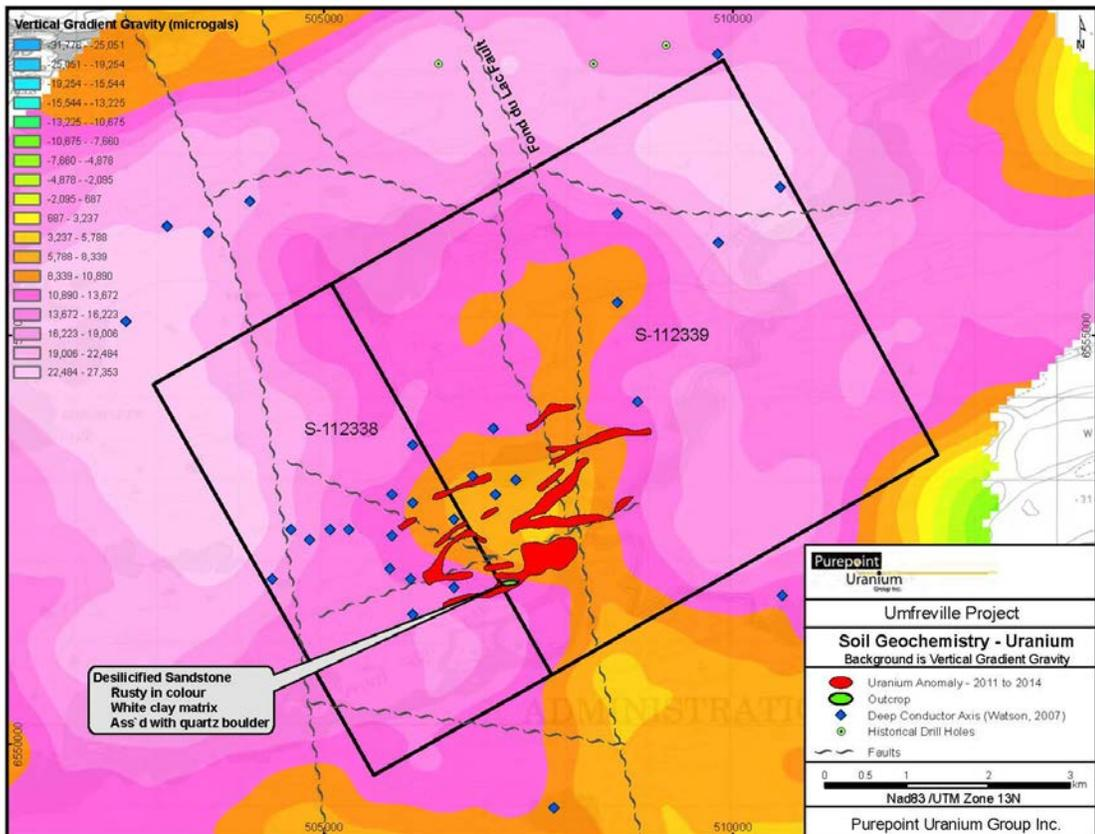
Figure 15: Uranium Soil Anomalies with Gravity Background
