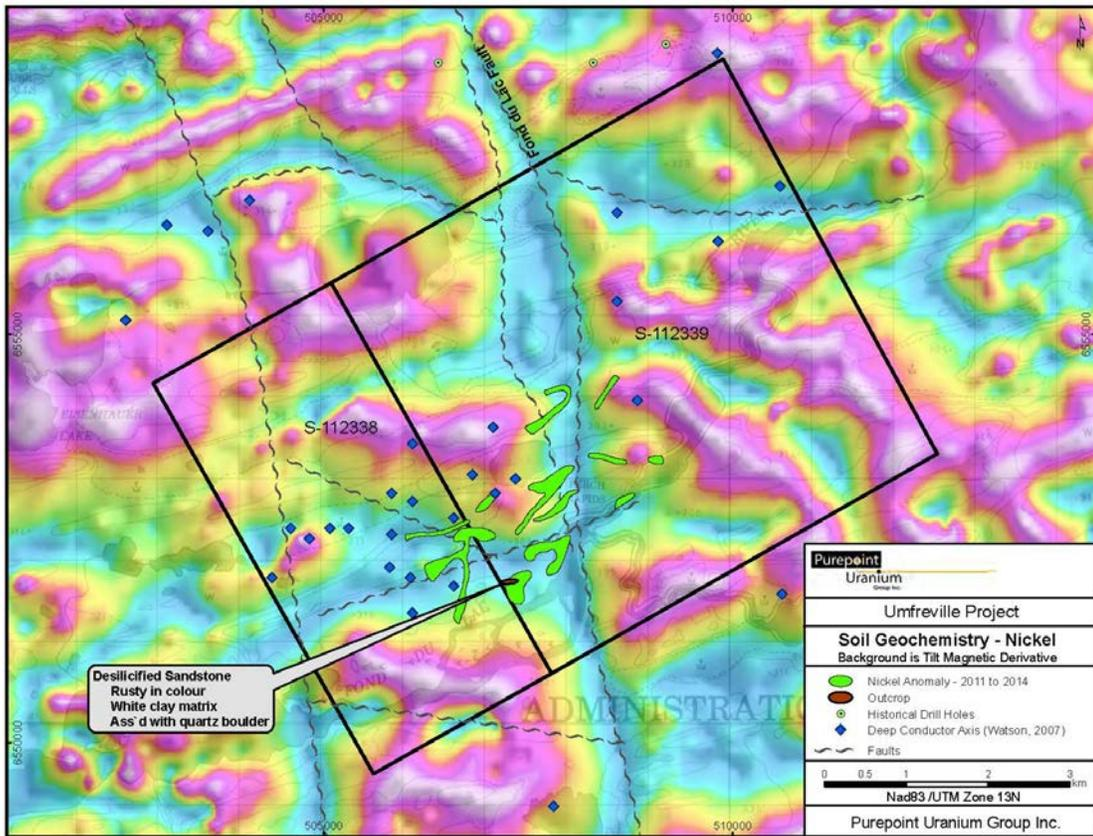
Figure 16: Nickel Soil Anomalies with Magnetic Tilt Derivative
