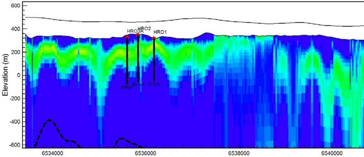
Figure 9: Example of LEI Resistivity Section showing Historic Drill Holes
