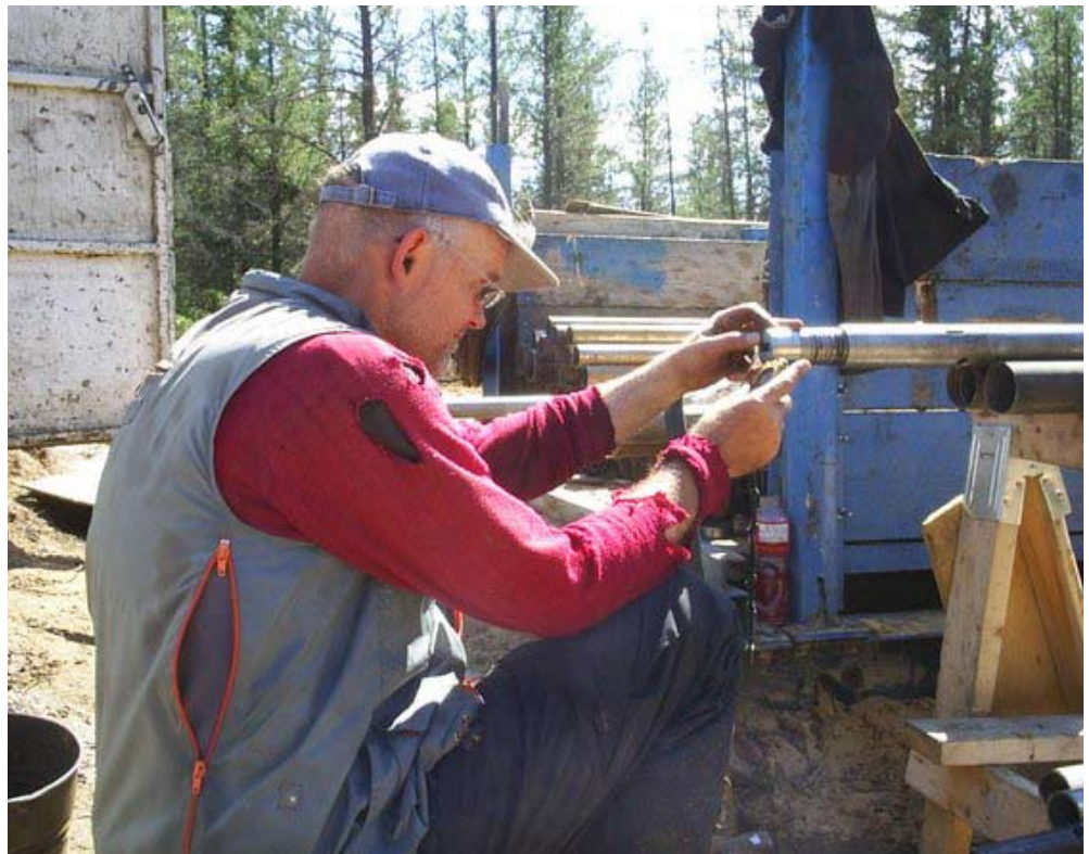
Purepoint Uranium senior geologist Peter Daubeny adjusts a core orientation tool at the Red Willow project drill site.
