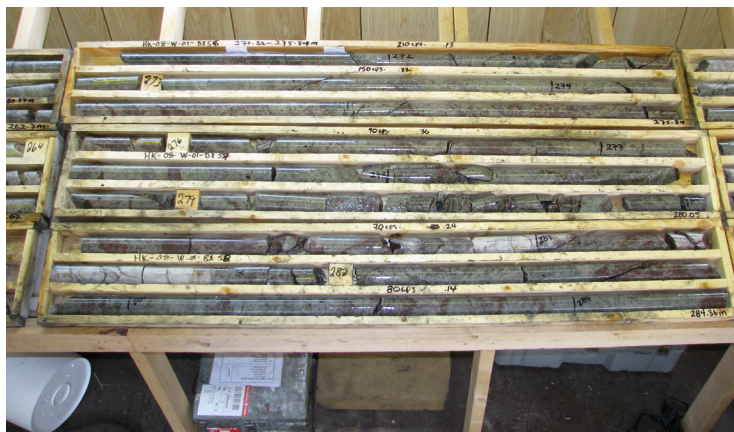
Figure 4: Core photo of HK08-03 showing strongly hematized and silicified basement rock 30 to 45 metres below the unconformity
